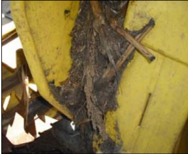
Soil contamination on used forage harvester imported from Argentina.
