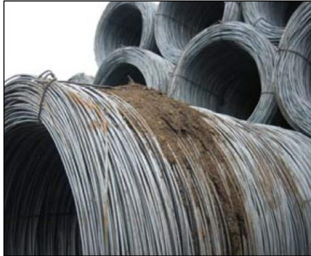
Soil contamination on imported steel coils.
